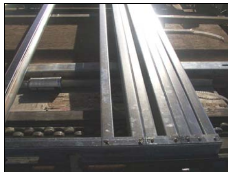
Example of multiple studs that hinder access for clinching.
