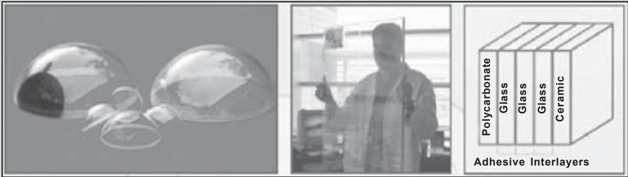
From left to right: 1) Transparent ceramics for sensor windows 2) Sapphire-based transparent armor prototype 3) Vehicle transparent armor windshield laminate system
