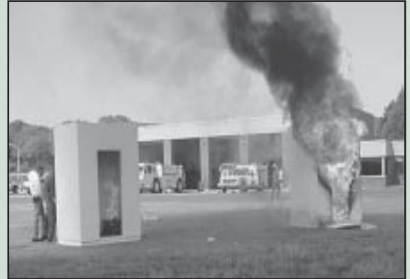
Demonstration of Intumescent paint product, Firefree 88®, in San Francisco.
